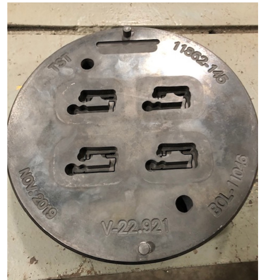
The aluminum extrusion die design examined in this case study.
